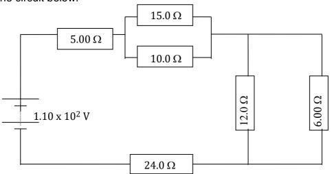
(a) Calculate the total resistance of the circuit.
