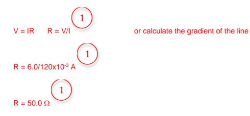
(d) Calculate the resistance of the filament light bulb when the voltage is at 8.00 V.
